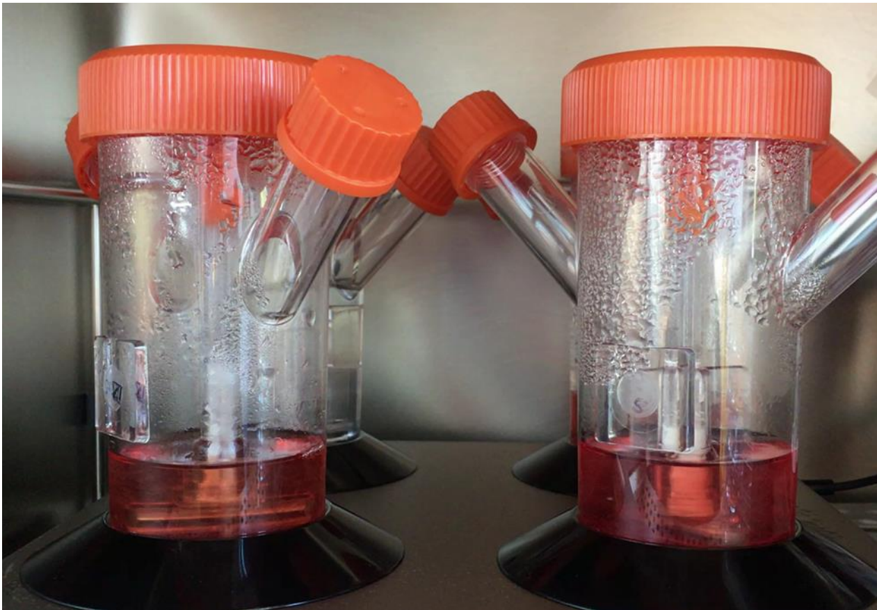
FIG 1. Example of commercially available Corning spinner flasks (125 ml) in a culture stove. Spinner flasks are inoculated with 2.5 million cells in a 25 ml starting volume (expansion media) with 10% (v/v) Matrigel. Every other day media is added, and cells are cultured for a duration of two weeks. Rotation speed of the spinner flasks is 80 rpm.
